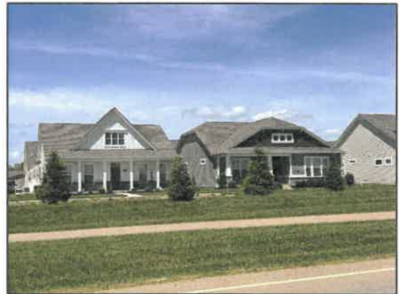
Figure 1: New housing development in the Dayton region utilizing a combination of cementitious siding, wood, and stone veneer. Note that the homes have attached garages, accessed from the rear.
